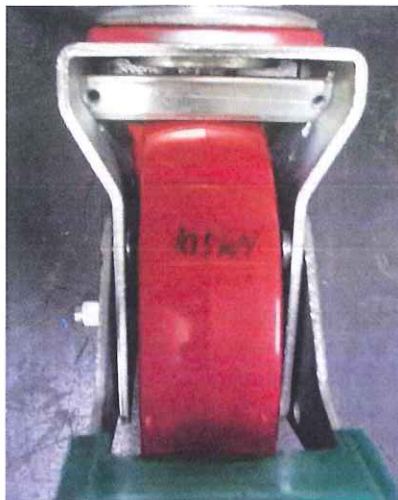
Figure 2: The depressions on the wheel after the application of the load. The load applied for the impression shown is marked on the photograph: 10.5kN for 1.5 times the rated load and 21.0kN for 3 times the rated load
