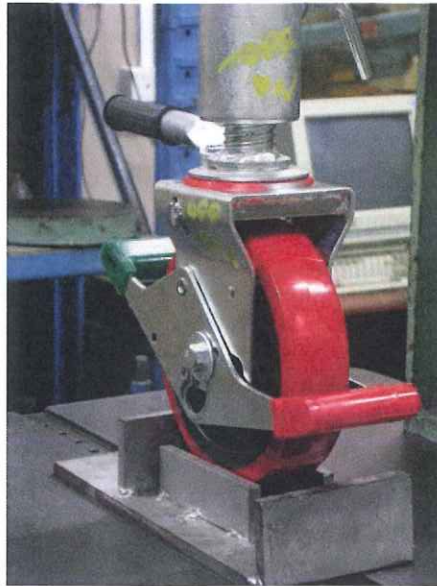
Figure 1: The loading of the castor in the test machine
